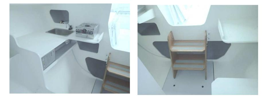
The inside has been polyester Flo-coated white, applied with a mohair roller. If any modifications need to be made or additions laminated on, the polyester flo-coat will be easier to prepare than grinding paint back to the fibreglass.
