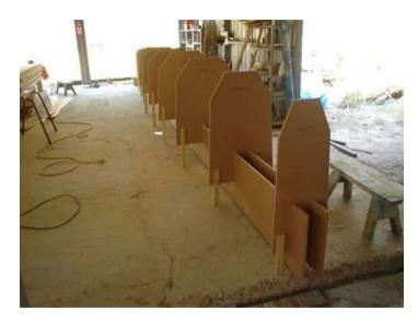
The panels were then attached to the temporary bulkheads using screw (for foam) or wired together (plywood).
