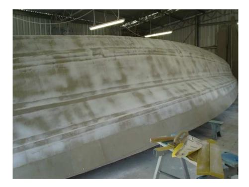
Once the boat is taped or glassed then the whole hull is filled and faired.
