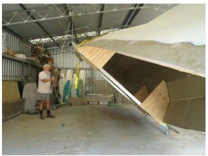
After the hull was turned over the joints were taped.
