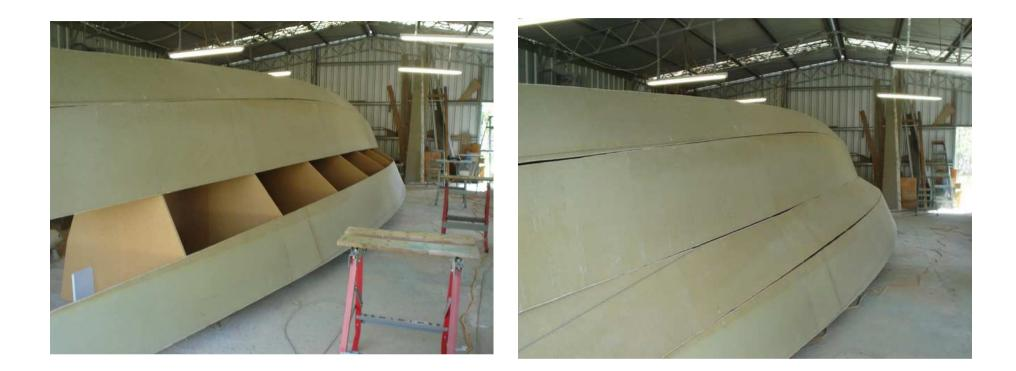
When all the panels are attached bog between the joints and sand. The joints can then be taped with glass tape (covered with peel ply. If the boat is plywood then the boat can be covered with glass and peel ply. The stem is clamped as the float and glued and taped.
