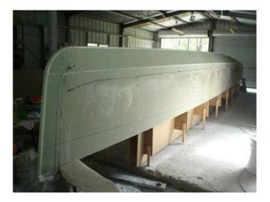
The float is turned and joints taped on the inside (pre-laminated panels) or glassed overall (plywood). It is easier to tape the inside joints using a wet fillet before taping.
