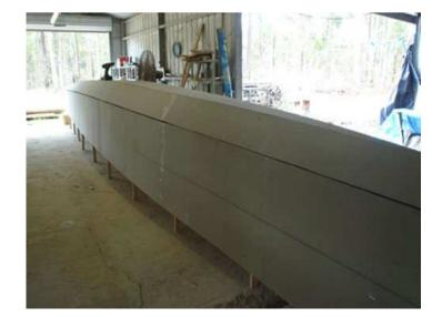
The stem of the float is clamped together and bog is applied to all joints.
