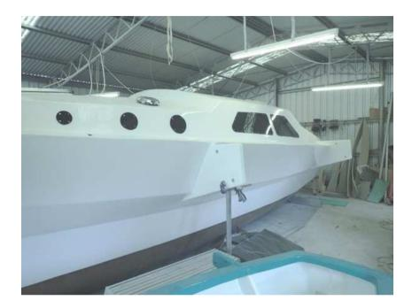
To move the main hull out of the shed it needed to be laid over on a trolley so it can pass through a 3metre wide opening. The trolley is made using 75x75x3 square hollow section steel on large castor wheels strong enough to handle the weight.
