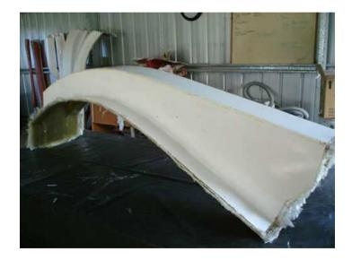
The beam flanges are trimmed and the beam is ready to be installed in the floats.
