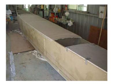
The deck was taped to the float. All joints were sanded and float was filled ready for paint.
