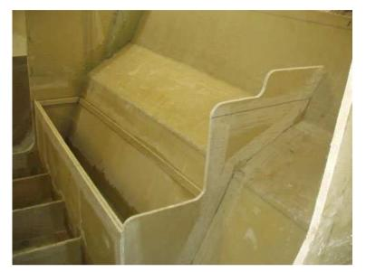
Horizontal shelves to the sides were added for a navigation station and a shelf for the portable fridge and platform for the porta-potti.
