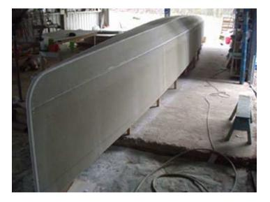
The joints are sanded and taped (if using pre-laminated panels) or glass over-all if using plywood. Taping the joints using fibreglass tape and resin. If the joint will be in an area to be finished then you can use peel ply. This will make finishing much easier. The bottom panel and the bilge panels are covered with an additional layer of double bias glass and peel ply to protect the bottom of the float.
