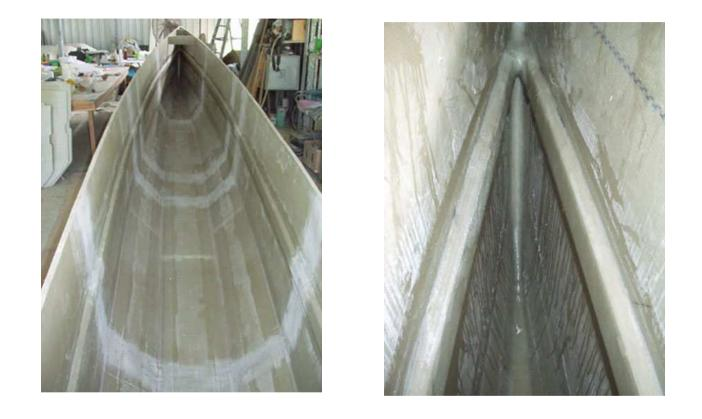
The bulkheads are temporally held in place and taped. A couple of deck beams are added to support the deck.
