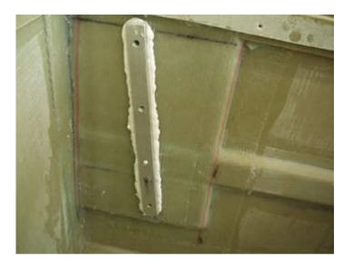
Glue was liberally spread on top of bulkheads, deck beams and in-wales. Deck was added using metal strapping to hold it in place.
