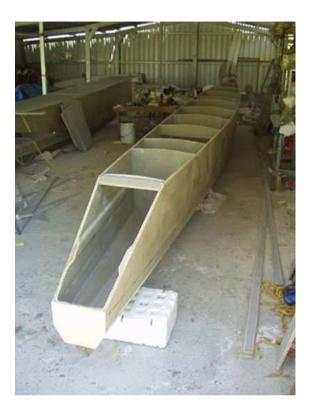
The transom is cut and added. In-wales were glued and clamped to support the deck.
