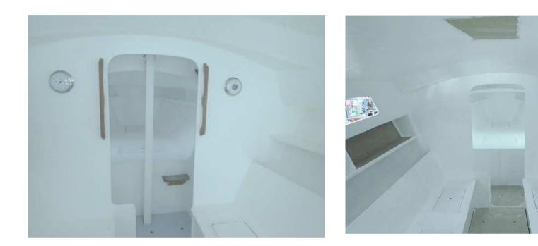
The cockpit was built with number 4 and number 6 bulkhead used as supports for the cockpit seats.
