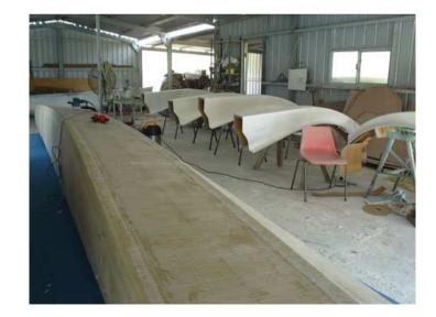
The floats were primed and anti-fouled ready for the beams to be added.
